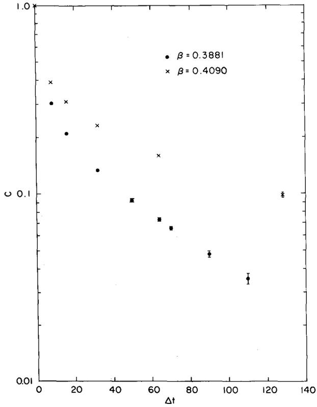
FIG. 5. The temporal correlation of a spin with itself as a function of the time between measurements. The solid points represent a lattice with  $\beta = 0.3881$  and the crosses,  $\beta = 0.4090$ .
